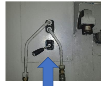
Gently lift up the "Lever" to lift up the bin.
