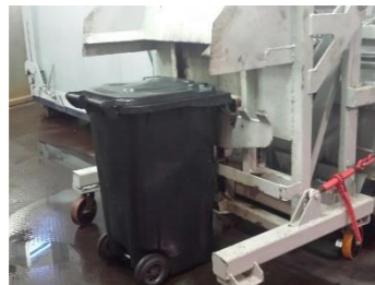
Kindly wait for 10 seconds for oil to run, then gently pull down the "Lever" to bring down the bin.
