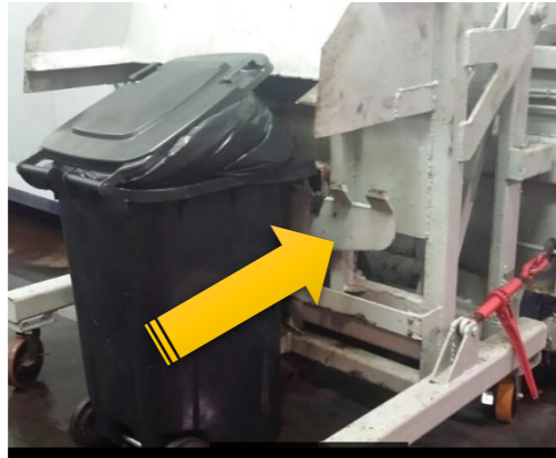
Push in the 240- litre bin or 660-litre bin into the lifter
