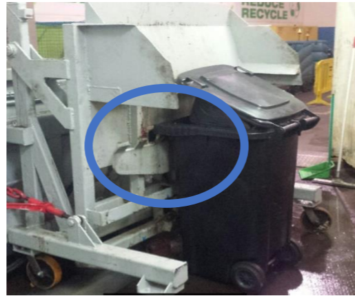
Hook up the bin and ensured that it is properly secured to the lifter
