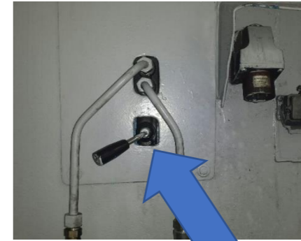
Kindly wait for 10 seconds for oil to run before using Lever to operate the Bin Lifter
