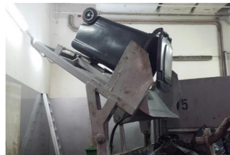
Hook up the bin and ensured that it is properly secured to the lifter
