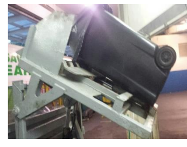
Gently lift up the "Lever" to lift up the bin.
