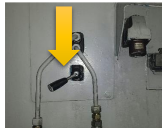
Kindly wait for 10 seconds for oil to run, then gently pull down the "Lever" to bring down the bin.
